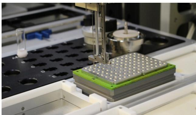
Figure 7: The Big Kahuna automatically dispenses the required amount of solvent to the plate.
