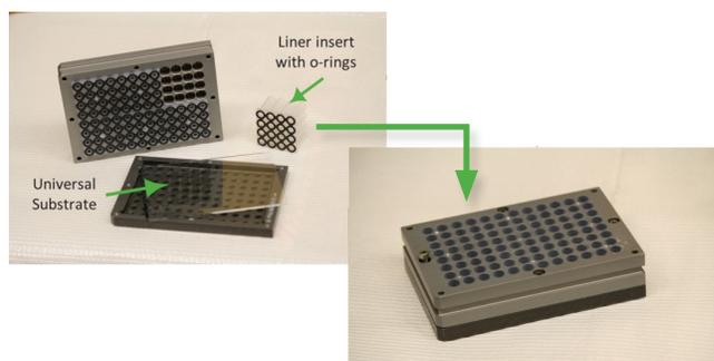
Figure 4: The crystallizer assembly is composed of a 96-well plate, a glass or quartz plate (universal substrate) and disposable liner inserts. The steel balls and the compounds will be deposited in the liner insert. O-rings at the bottom of the insert will ensure that the material in each well remains isolated. The cocrysal will be formed on the universal substrate, which can be removed for analytical testing without further manipulation of the cocrysal.
