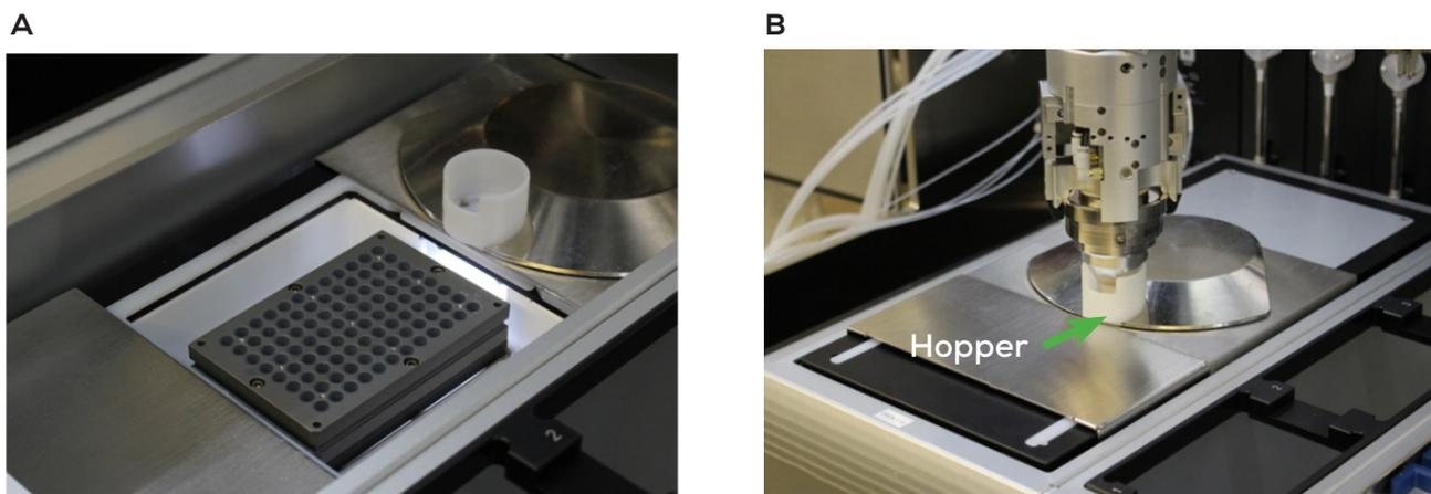
Figure 6: (A) The deck of the Big Kahuna with the crystallizer assembly in the on-deck balance. (B) The solid dispensing arm with hopper containing powder to be dispensed.
